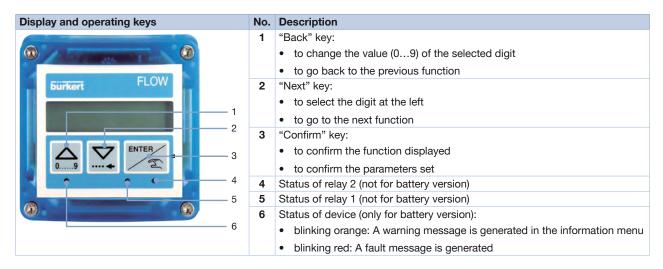
The device can be calibrated by means of the K-factor of the sensor-fitting used, or via the Teach-In function. User adjustments, such as engineering units, output, filter, bargraph are carried out on site.
